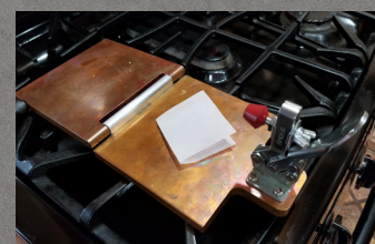
FIGURE 4 Place material in parchment paper onto the bottom plate.
