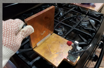
FIGURE 3 While wearing gloves, lift handle and open the top plate.
