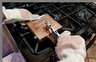
FIGURE 5 Wearing BOTH gloves, close top plate and apply clamp until it clicks. Leave material clamped for 8- 10 seconds. USING GLOVES, unclamp and open top plate. Remove the parchment envelope immediately so as not to burn or overheat your material.
