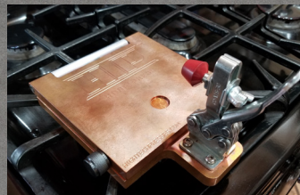
FIGURE 1 With clamp in the open position, place Press on burner over a medium flame or heat for approx. 5 minutes. Make sure flame does not protrude out the sides.
