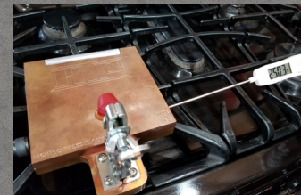
FIGURE 2 Insert digital thermometer shaft into the hole opposite of handle. When desired temperature is achieved, turn the flame/heat off.
