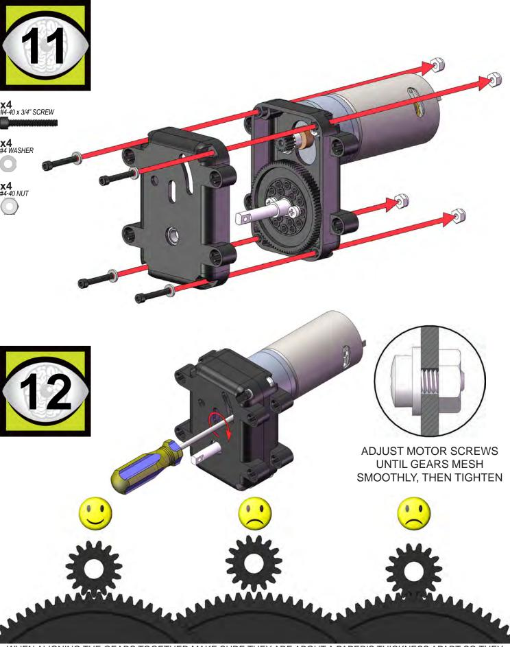
WHEN ALIGNING THE GEARS TOGETHER MAKE SURE THEY ARE ABOUT A PAPER'S THICKNESS APART SO THEY MESH SMOOTHLY. DO NOT LEAVE THEM LOOSE OR PRESS THEM TOO TIGHT TOGETHER OR IT MAY DAMAGE THE GEARS OR PUT TOO MUCH STRESS ON THE MOTOR.
