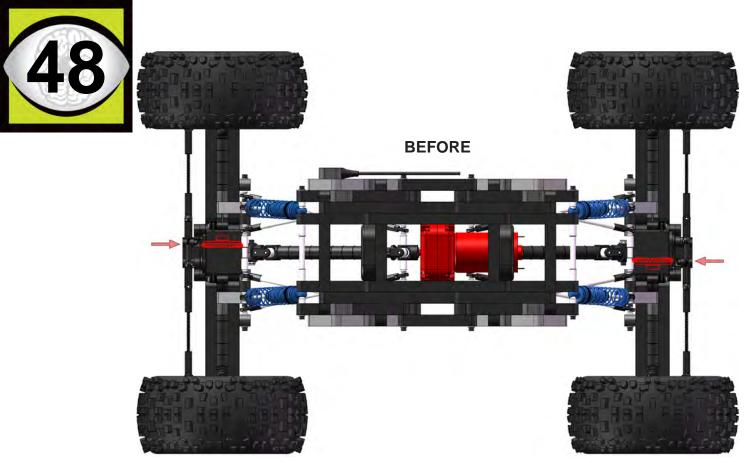
DUE TO THE SECOND MOTOR CASE REVERSING THE ROTATION OF THE FRONT DRIVELINE, THE FRONT DIFFERENTIAL NEEDS TO BE "FLIPPED". DURING ASSEMBLY BE SURE TO HAVE ONE AXLE WITH THE RING GEAR ON THE LEFT, AND THE OTHER ON THE RIGHT AND THEN INSTALLED ACCORDING TO THE DIAGRAM BELOW. IF YOUR KIT IS ALREADY ASSEMBLED, SIMPLY REMOVE THE FRONT CENTER HOUSING AND FLIP THE DIFFERENTIAL UPSIDE-DOWN AND RE-INSTALL.
