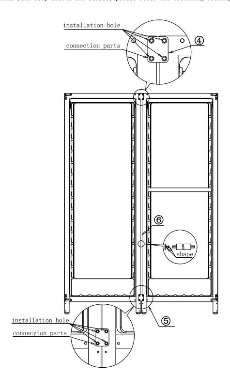
6. To install 2 in 1 stainless steel ventilation plinth, fix the cross-head screw on the plinth with phillips screwdriver; (please refer the following drawing?)
