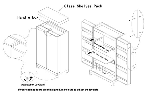
on the bottom of the feet until the doors are flush and properly aligned
