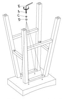
Attach the assembled leg set to the wood seat using Bolts (A), Lock Washer (C), and Flat Washer (D).
