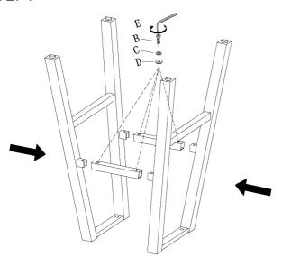
Attach both side runners to the legs using Bolts (A), Lock Washer (C), and Flat Washer (D).
