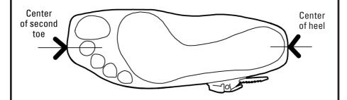
Center the skate frame on the center of your heel at the back and center of your 2nd toe at the front
