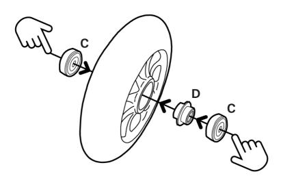
Once all wheels have 2 bearings (C) and 1 spacer (D) per wheel, one at a time align the bearing hole up with the axle hole on the frame
