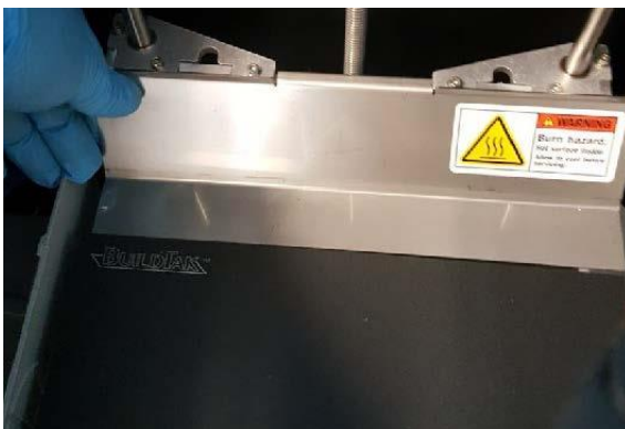
Figure 8) Z-Carriage barrier placement
