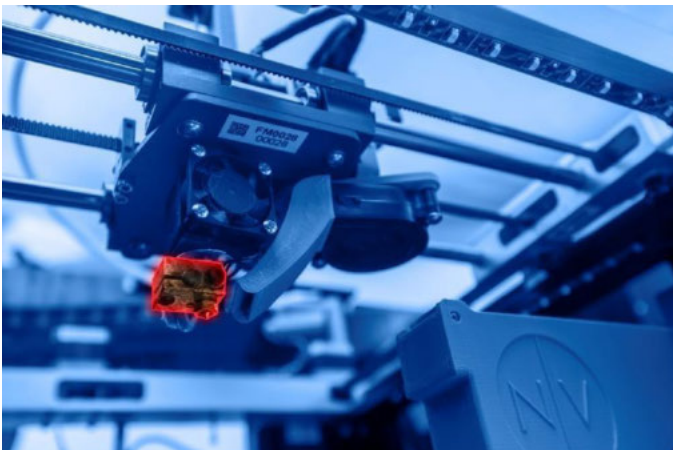
Figure 14) Hot-end burn hazard
