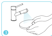
Wash Microfiber filter in running water.
