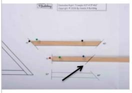
To measure and cut the **next** side of the triangle, align the end of your wood strip with the 90-degree angle on the blueprint. **Note:** Use the miter box to cut off the end tip of the wood strip at a **90-degree angle.** Pin the strip in place.
