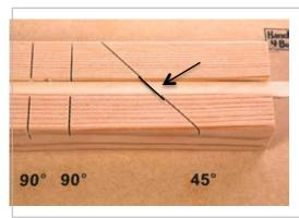
Align the 45- degree angle pencil mark on the wood strip with the 45-degree angle saw guide on the **right** side of the miter box.
