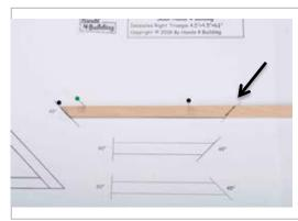
Align the 45-degree angle on the wood strip with the 45-degree angle on the blueprint. Place 2-3 pins in the foam core board at the edge of the wood to secure the strip.
