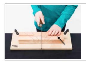
Fingers on your free hand will hold the wood strip in place in the miter box slot while you cut the strip with the saw. Keep fingers at a safe distance from the saw blade.
