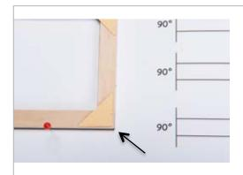
Glue **one half** a yellow triangle at every joint for added reinforcement. Place the glue on one side of the yellow triangle. Align the triangle with the edge of the wood.
