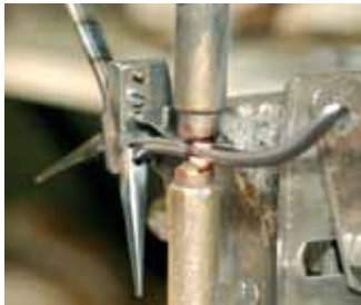
Spot-welded fixed position double leaf springs
