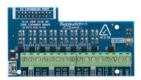
The CM707B Plug On Zone Expander is designed to complement the CM705B Universal Zone Expander. It can be added via the expansion port on the CM705B Universal Expander to provide an additional 8 hard wired zone inputs, bringing the CM705B to 16 hard wired zone inputs for Alarm + Tamper, 4 state monitoring or Single EOL configurations.
