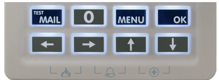
Figure 22: Keypad Emergency Alarm Trigger's
