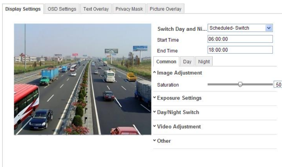
Figure 6-32 Day/Night Scheduled-Switch Configuration Interface
