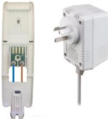
The DB7 requires 1A and 12 volts at the DB7 connection terminals over the supplied wires. Make sure the wires support this power. Connecting to the AUX terminals of the alarm panel will not receive enough current needed for correct operation.
