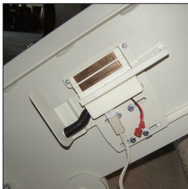
6. lower charge contact no final limit (back of rail)
