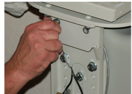
Loosely secure with 2 bolts.
