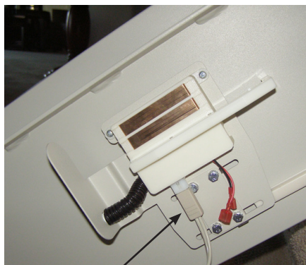
charger connection to charge contact
