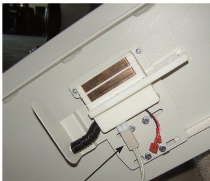
charger connection to charge contact
