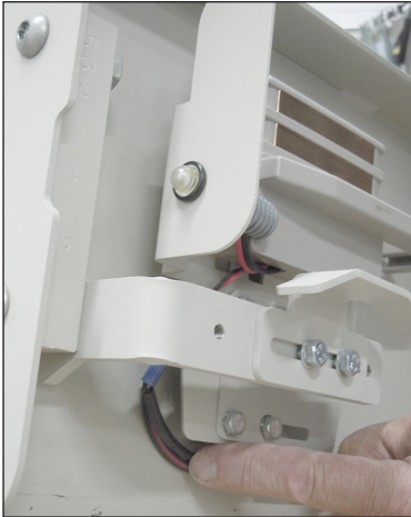
5. upper charge contact tuck wire connections (back of rail)
