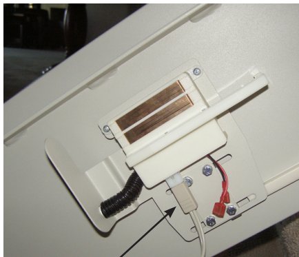
charger connection to charge contact
