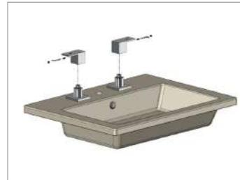
4. Position the spout to the center of the hole and mount to assembly breach. Tighten all fittings and test for leaks.
