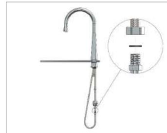
4. Adjust the counter weight now to ensure the hose will retract correctly, then tighten. Connect the flexible hoses to the isolating stop cocks (check that as the hoses are being tightened that they are not loosening on the mixer body). Test for leaks.
