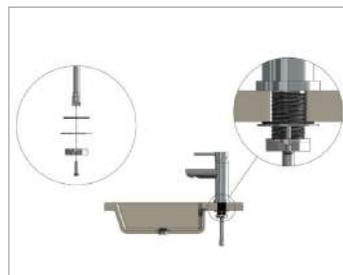
4. Connect the flexible hoses to the isolating stop cocks (check that as the hoses are being tightened that they are not loose from the mixer body). Test for leaks and correct operation of the mixer.
