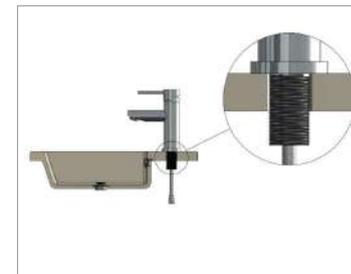
3. Place the rubber washer (part 2) over the flexible hoses and push up until it is firm against the surface being mounted on, then push (part 3 + part 5) the fixing plate and fixing nut over the flexible hoses and tighten firmly and tighten screws where applicable.
