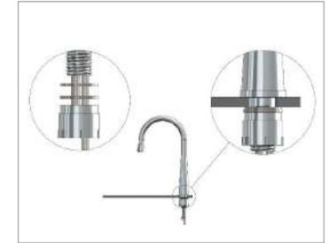
3. Attach the counter weight to the pull out flexible hose (part 2) **DO NOT TIGHTEN** (as the counter weight will need to be adjusted later on). Connect the flexible hoses and tighten (part 7) to the water outlet ensuring the rubber seal is not missed.
