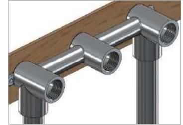
3. Now install the wall tops and insert a 1/2-inch male BSP threaded pipe into the center outlet using threaded tape or plumbers tape (not provided) ensuring all the fittings are tight and tested for leaks and operation. Apply clear sealant if required.
