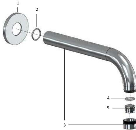
1. Apply thread tape to the exposed G1/2" BSP thread, ensure the back plate (part 2) is installed on the body of the spout before screwing the spout clockwise (by hand) onto the G1/2" BSP thread (the spout should finish up tight against the finished surface).
