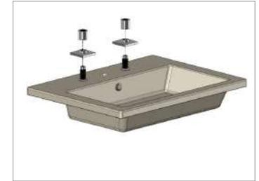
3. Install the handles and tighten the grub screw (ensure the spindles are turned to the off position and the handles are aligned correctly before tightening the grub screw).
