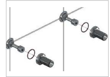
3. Slide the cover plate and fixing nut over the spindle and hand tighten (if there is not enough thread to tighten the fixing nut on you will require extended spindles or spindle extensions, these can be purchased separately).
