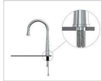
2. Place the rubber seal (part 2) over the flexible hoses and push up until it is firm against the surface being mounted on, then push (part 5 + part 6) the fixing plate and fixing nut over the flexible hoses and tighten firmly.
