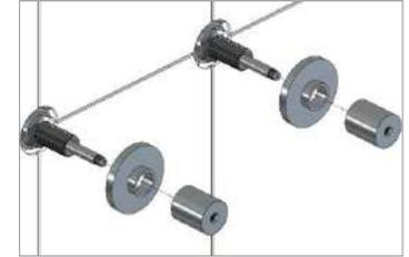
3. Install parts 4, 5 and 6 then tighten accordingly. Use care when using the provided 2 prong spanner to avoid scratching the spindle. Test for leaks around the spindle bodies and to ensure the wall tops are functioning correctly.
