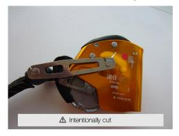
ASAP LOCK prototype after dynamic test
