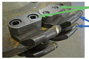
Tomahawk bolts can be installed from whichever side of the wheel you have better access to.
