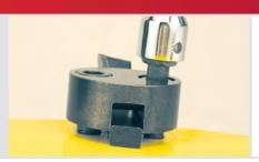
**Why?** Due to the heat treated pocket which allows the pocket to clamp the tooth when tightened and then when loosened it springs open to allow the tooth to easily slide out for removal.
