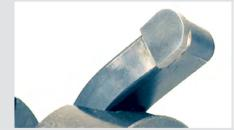
**Why?** This strength comes from the 3/4" shank and its precision fit to its heat treated pocket; the combination of the two give it its superior strength.
