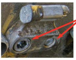
This brand requires you to have access to both sides of the wheel all of the time in order to install the teeth. This requires you to jump back and forth from one side of the wheel to the other in order to take a pocket off.
