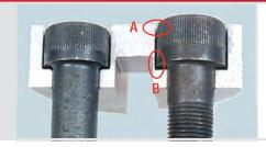
**Why?** Shorter Head height creates the added recess in the pocket and this protects the bolt head from being damaged when the pocket begins to wear. The smaller diameter to create a smaller counterbored hole so we can make the pocket walls thicker.
