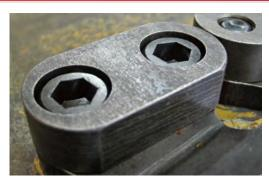
Tomahawk bolts are recessed and protected within the mounting block which allows teeth to be removed and changed faster and with less effort.
