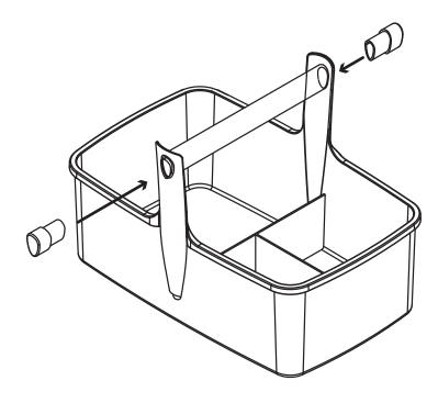
To assemble, align Carrying Handle with holes in vertical posts of Caddy. Once aligned, insert End Caps to hold in place.
