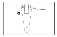
**Step 3:** Move brackets away from wall and drill a hole in the marked areas, using 1/4" drill bit.
