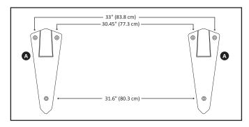
**Step 4:** Using a level, make sure the brackets are fully aligned. Once aligned, tighten brackets securely in place.
