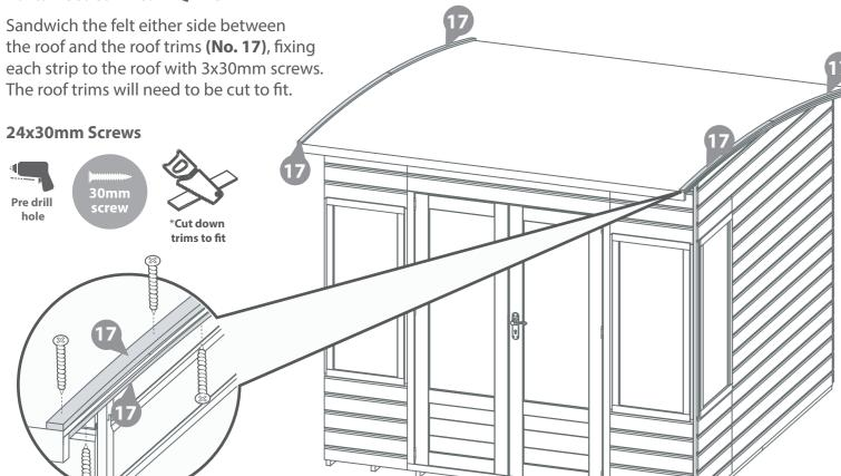
IMPORTANT: Pre-drill before fixing screws.
