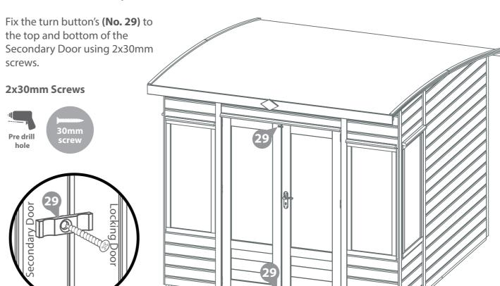
\*These turn buttons help keep your doors straight during high and low levels of moisture content in the air.
