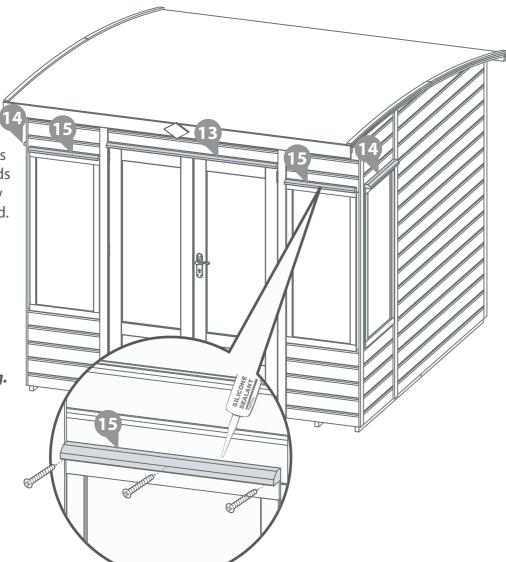
IMPORTANT: Pre-drill before fixing screws.
