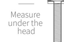
To identify the fixings required for each step use a measuring tape.
