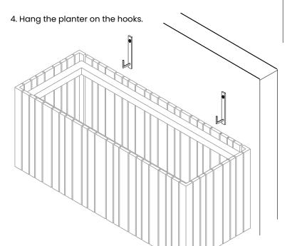
5. The hooks should be fitted in between two planks and below the upper construction frame.
