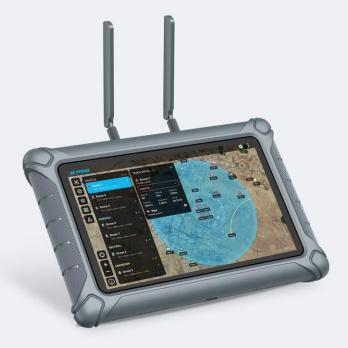
Guider C2 software offers an intuitive and feature-rich software platform, providing C-UAS awareness and reporting capability. Supported by sensor fusion, computer vision, edge computing, machine learning and artificial intelligence, Guider integrates radars, detectors and jammers, consolidating their data into a display. It is always on alert, ensuring round-the-clock monitoring of drone threats and effectively mitigating human error.
