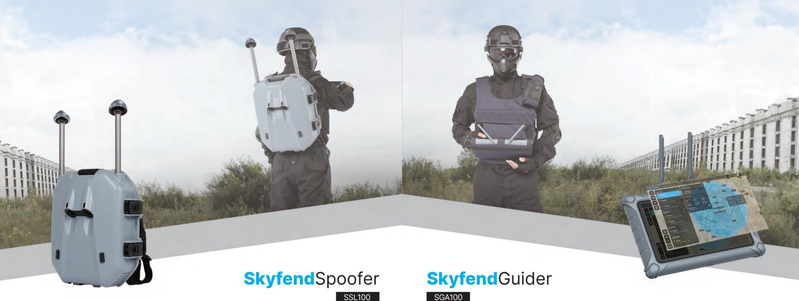
Spoofer is an advanced GNSS navigation spoofing device engineered explicitly for SUAVs. Its primary purpose is to enforce area denial, redirect drones to predetermined orientations and manipulate their flight paths to designated locations. When combined with radar, spectrum detection devices and jammers, it can cause drones to crash or force them to land at appointed locations.
