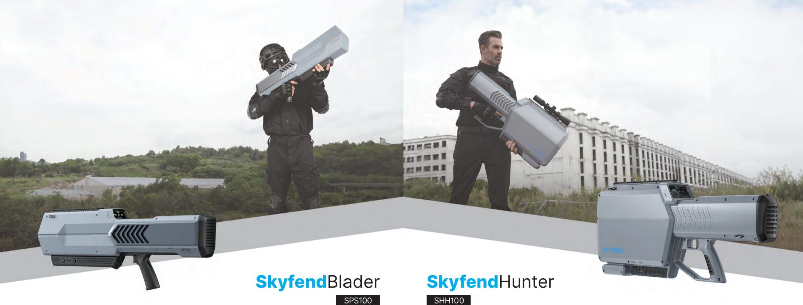
Blader is a portable jammer for SUAVs. Featuring countermeasures for UAV flight control, map transmission, and GNSS bands, it can repel drones or force them to crash to solve the threat of roque SUAVs.
