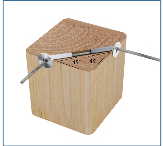
Option 2: An adjacent pre-drilled post to go with 2 protector sleeves CR69 to bear force and let the cable go through the corner. The size of corner post must no less than 4" x 4".
