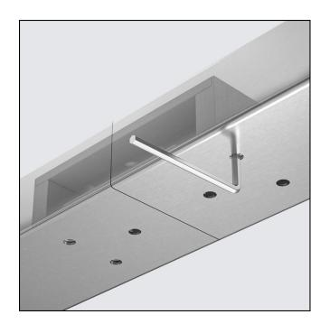
**Step 3 -** Tighten the set screws **9** until the connector **8** is completely tapped in handrails.
