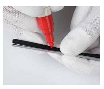
**Step2 -** Mark the depth of terminal on the wire rope.
