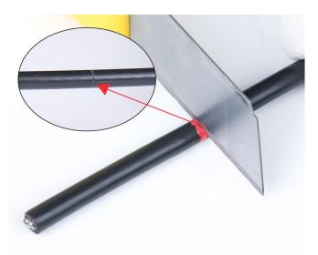
**Step3 -** Ring-cut the vinyl coating along the mark.
