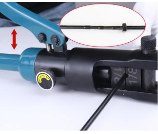
**Step6** - Crimp the 1/8" terminal with the bare wire rope.
