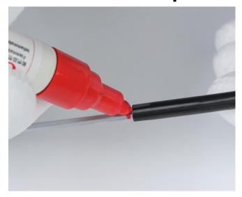
**Step1** - Measure the depth of the 1/8" terminal by a thin rod or something similar that can be inserted into terminal; and mark the depth on the rod.
