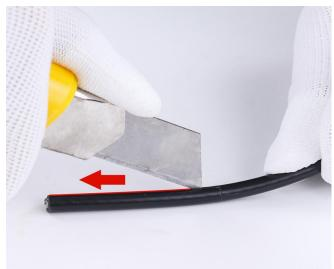
**Step4** - Cut the coating along the wire rope.
