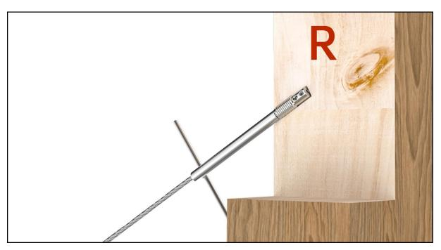
**Step 10 -** Tighten the tensioner **10** with the socket wrench **9** on the right post.
