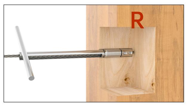
**Step 10 -** Tighten the tensioner **1** with the socket wrench **9** on the right post.
