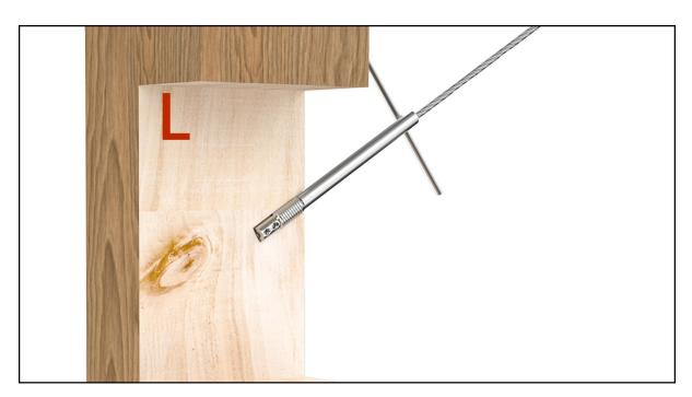
**Step 6 -** Tighten the tensioner **1** with the socket wrench **9** on the left post.
