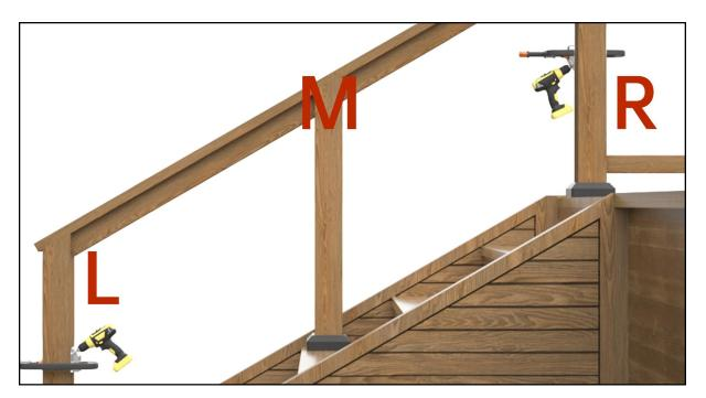
**Step 3 -** Drill 30 degrees 2 3/8" deep holes with drill guide 8 on the right and left posts with a 13/32" drill bit.
