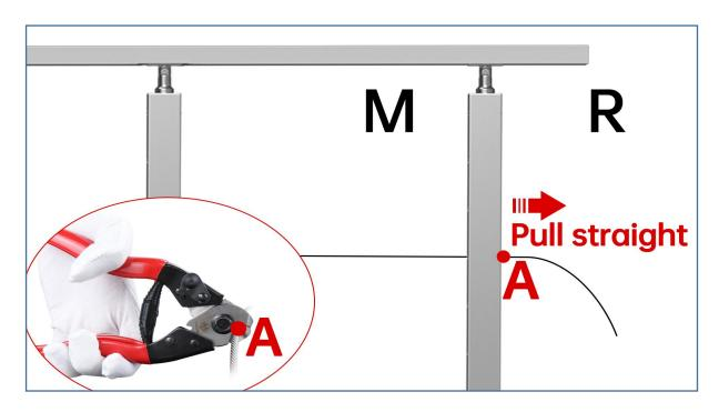
**Step 4 -** Pull the cable against the right end post, mark point A from the outside of R post, and cut cable on point A with cable cutter **6**.
