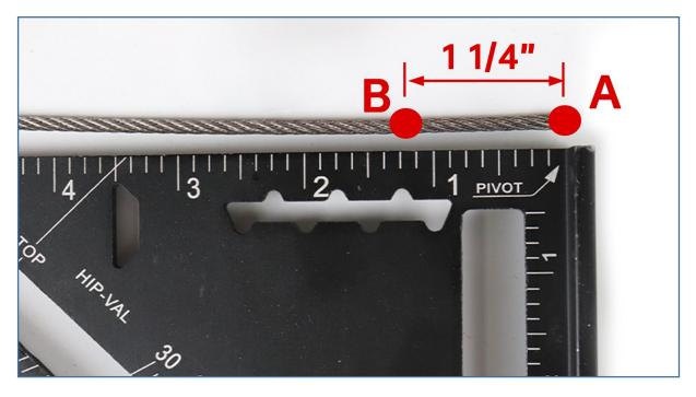
**Step 5 -** Mark and cut at point B with cable cutter **6**, which is 11/4" away from point A.
