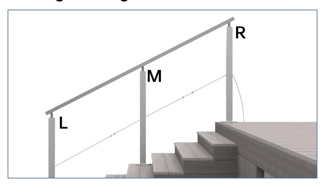
**Step 1 -** Pass cable from the right post to the left post, put in adhesive washers **7** for both L&R posts, and angle protector sleeve **8** for middle posts.
