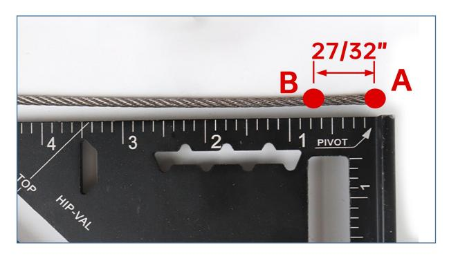
**Step 5 -** Mark and cut at B, which is 27/32" away from point A, with cable cutter **6**.
