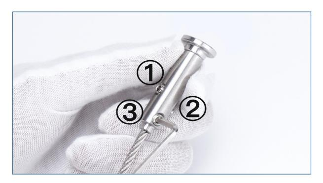
**Step 6 -** Put the cable into the tensioner **1** and tighten the set screws in sequence with the 2.5mm Allen wrench **3**.
