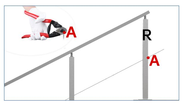
**Step 4 -** Pull the cable against the right end post, mark point A from outside of the right post, and cut cable on point A with cable cutter **6**.
