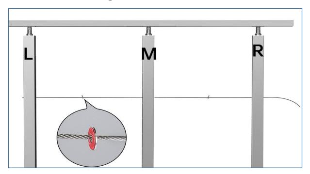
**Step 1 -** Pass the cable from the right post to the left post, put in adhesive washer **7** for both L&R posts .
