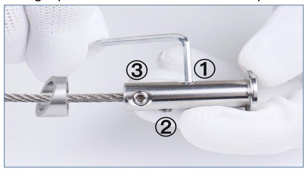
**Step 2 -** Put in angle washer **10** before tightening the set screws in sequence with the 2.5mm allen wrench **3**.
