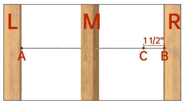
**Step 4 -** Measure two end posts span and mark point B on the cable, cut the cable at point B with cutter 7.
