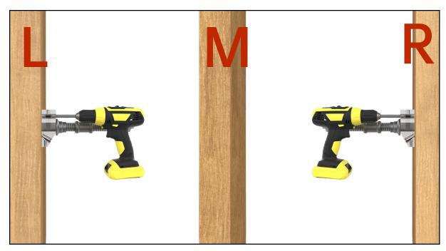
**Step 2 -** Locate the hole positions with drill guide **9**, and drill 2 5/32" deep holes with a 3/16" drill bit **4** on all end posts.
