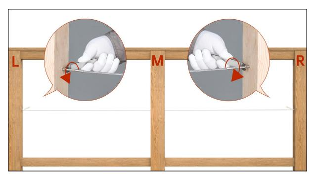
**Step 7 -** Use bent wrench **3** to tighten the left-hand lag screw **1** and right-hand lag screw **2** in the same direction on both end posts.
