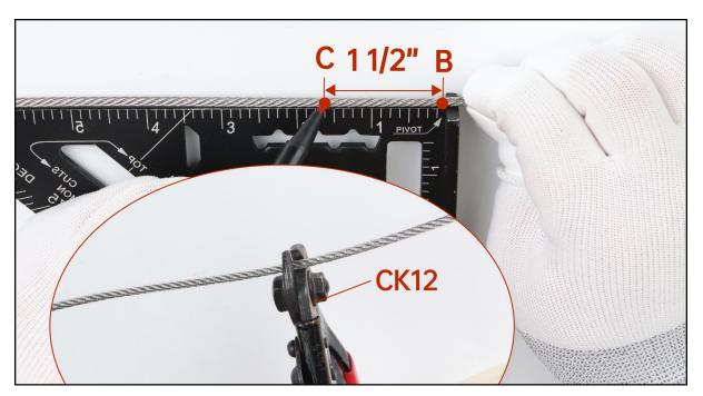
**Step 5 -** Mark and cut at C, which is 1 1/2" away from point B with cable cutter **7**.
