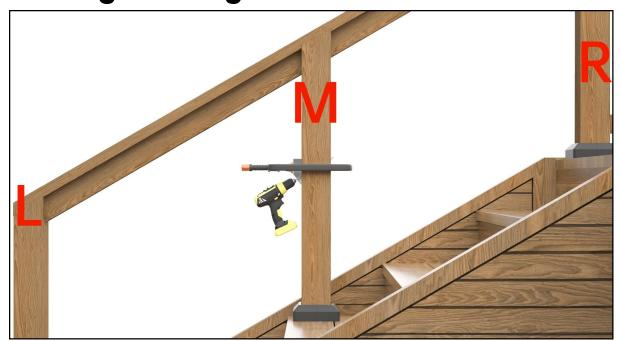
**Step 1 -** Locate hole positions, and drill 30 degrees through holes with a 5/16" drill bit **10** on intermediate posts.
