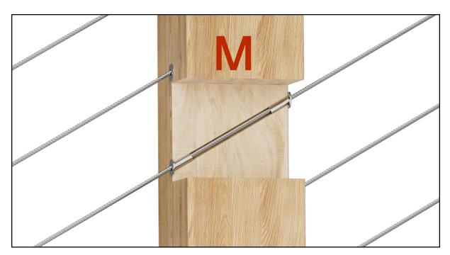
**Step 3 -** Pull cable **5** and angle protector sleeves **8** through all intermediate posts, then install these sleeves **8**.
