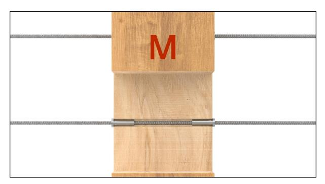
**Step 3 -** Pull cable **5** and level protector sleeves through all intermediate posts, then install these sleeves **6**.
