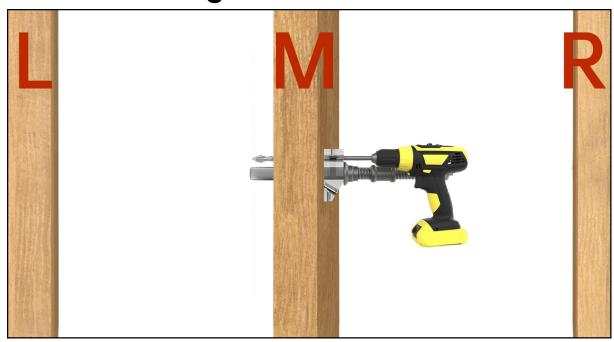
**Step 1 -** Locate the hole position with drill guide **9**; drill through holes on the intermediate posts with a 9/32" drill bit **10**.
