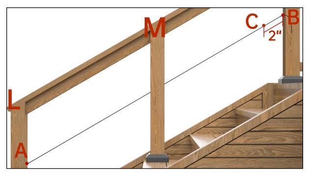
**Step 4 -** Measure the two end posts span and mark point B on the cable, cut the cable at B with cutter 7.
