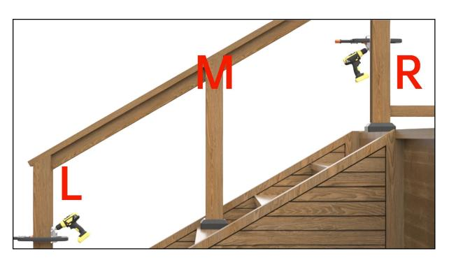
**Step 2 -** Locate hole positions with drill guide **9**, and drill 30 degrees 2 5/32" deep holes with a 3/16" drill bit **4** on all end posts.
