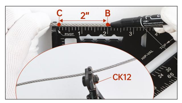
**Step 5 -** Mark and cut at C, which is 2" away from point B with cable cutter **7**.
