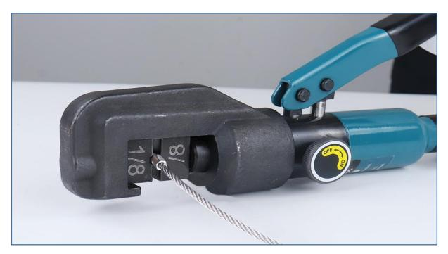
**Step 2 -** Swage the fixed end **1** with hydraulic crimper **4**.
