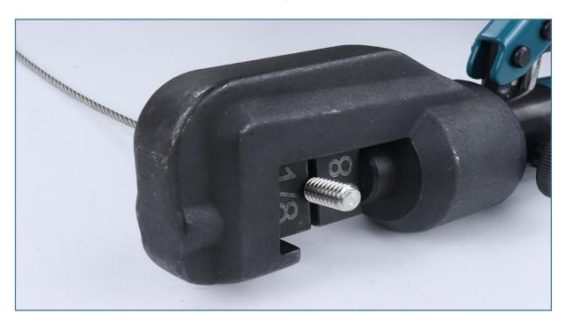
**Step 6 -** Swage tensioner **1** and cable with hydraulic crimper **4**.
