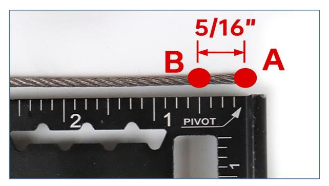
**Step 5 -** Mark and cut at B with cable cutter **4**, which is 5/16" away from point A.
