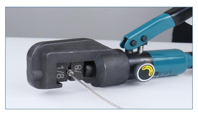
**Step 2 -** Swage fixed end **(1)** with hydraulic crimper **(4)**.
