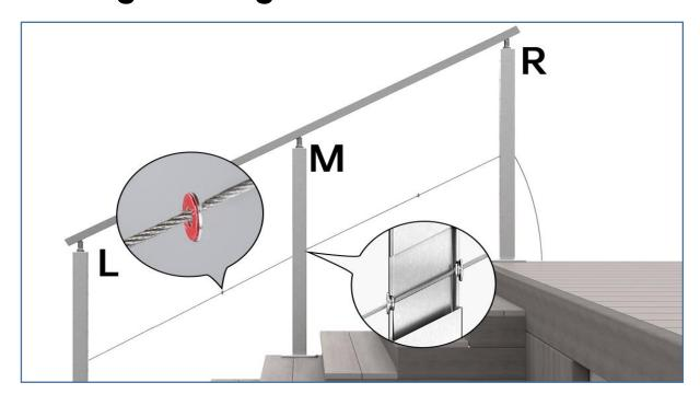
**Step 1 -** While pass the cable **3** from right post to the left post, put in adhesive washers **6** for end post and angle protector sleeves **9** for intermediate posts.
