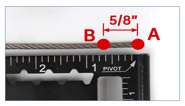
**Step 5 -** Mark and cut at point B with cable cutter 4, which is 5/8" away from point A.
