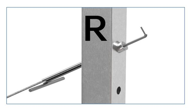
**Step 7 -** Put in angle washer **7**, tighten the tensioner with an allen wrench **2** and socket wrench **5** on the right end post.
