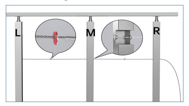
**Step 1 -** While pass the cable **3** from the right post to the left post, put in adhesive washers **6** for end posts and level protector sleeves **3** for intermediate posts.
