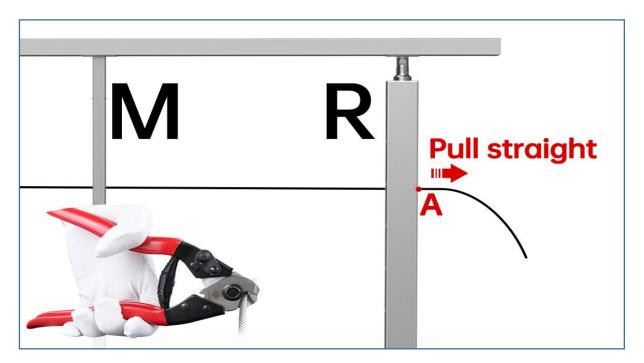
**Step 4 -** Pull the cable against the right end post, mark point A from the outside, and cut cable at point A with cable cutter **4**.
