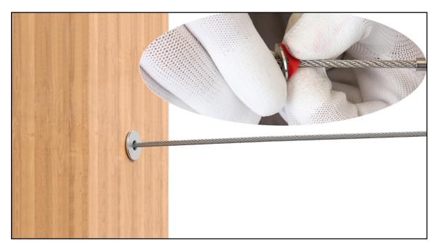
**Step 11 -** Install the adhesive washers **5** and level protector sleeves **7**.
