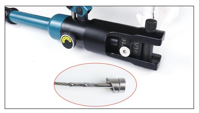
**Step 4 -** Put in angle washer **5** to the fixed end **1** before swaging with the hydraulic crimper **9**.
