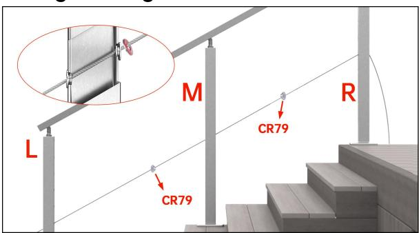
**Step 1 -** While passing the cable **2** from the right side to the left post, put in angle protector sleeves for intermediate posts.
