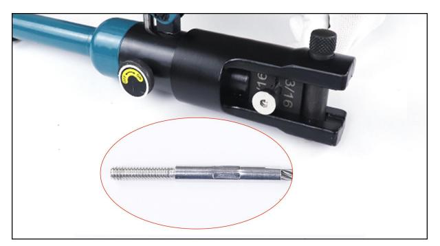
**Step 6 -** Swage tensioner **1** with hydraulic crimper **3**.
