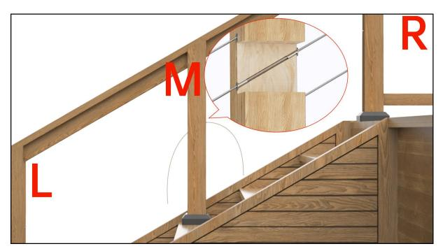
**Step 3 -** Put the adhesive washers **6** into the cable and pull the cable through all intermediates posts and angle protector sleeves **4**.
