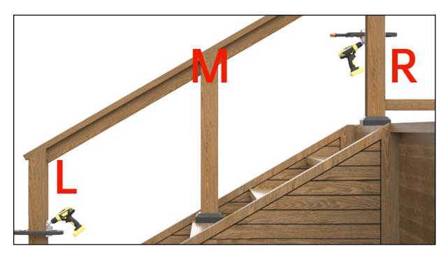
**Step 2 -** Locate hole positions and drill 30-degree hole with drill guide  $\bigcirc$ , drill through holes on the right post with a 13/32" drill bit, and drill through holes on the left post with a 5/16" drill bit.
