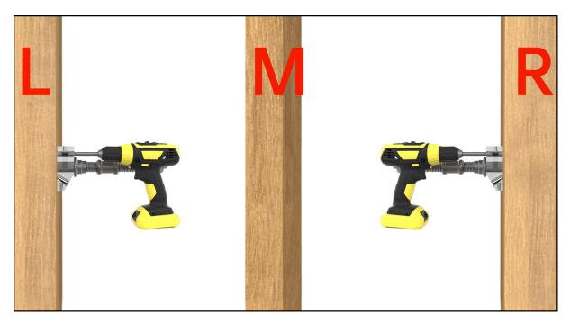
**Step 2** - Locate hole positions, drill through holes with drill guide on the right posts with a 13/32" drill bit, and drill through holes on the left posts with a 5/16" drill bit.
