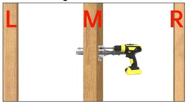
**Step 1 -** Locate hole position with drill guide 7; drill through holes on the intermediate posts with a 9/32" drill bit. (Note: please always keep 3" cable spacing when drilling).
