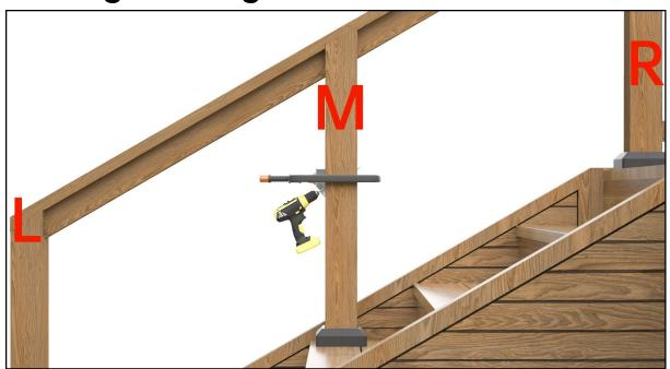
**Step 1 -** Locate hole positions and drill 30-degree holes with drill guide 7; drill through holes on intermediate posts with a 5/16" drill bit. (Note: please always keep 3" cable spacing when drilling.)
