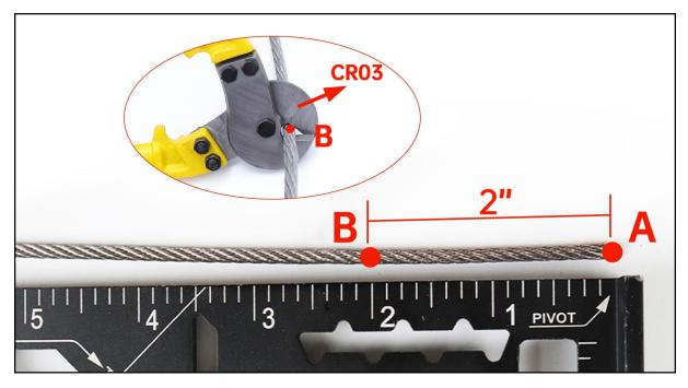
**Step 5 -** Mark and cut at point B with cable cutter **7**, which is 2" away from point A.
