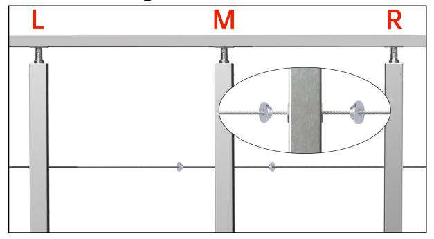
**Step 1 -** While passing the cable **2** from the right post to the left post, and put in level protector sleeves **5** for intermediate posts.
