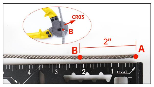
**Step 7 -** Mark and cut at point B, which is 2" away from point A with cable cutter **3**.
