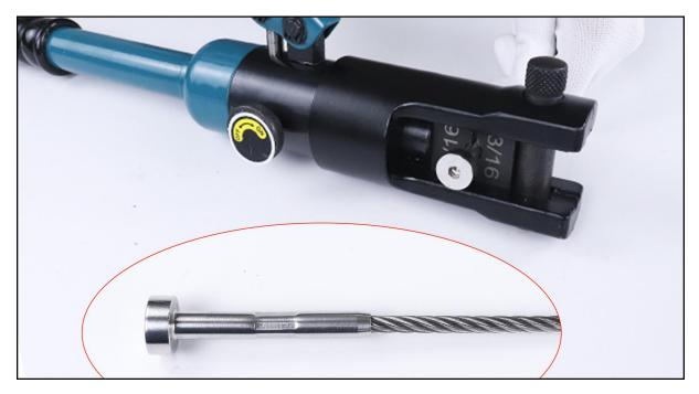
**Step 4 -** Swage the fixed end **1** with the hydraulic crimper **2**.
