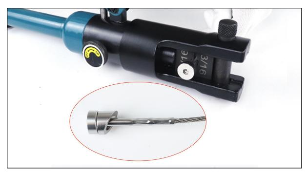
**Step 2 -** Put in angle washer **4** to the fixed end **1** before swaging with hydraulic crimper **8**.
