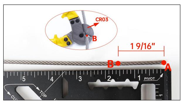
**Step 7 -** Mark and cut at B with the cable cutter **3**, which is 1 9/16" away from point A.
