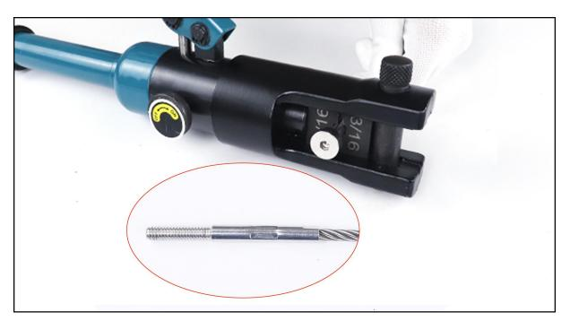
**Step 6 -** Swage tensioner **1** with hydraulic crimper **3**.
