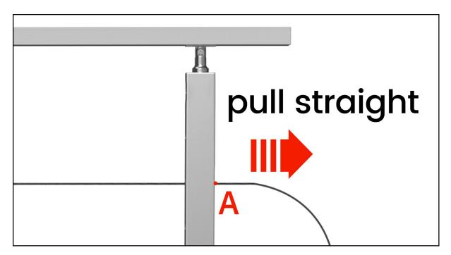
**Step 4 -** Pull the cable against the right end post, mark point A from the outside, and cut cable on point A with cable cutter **7**.
