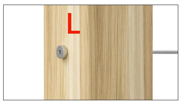
**Step 5 -** Install the fixed end **1** to the left end post.
