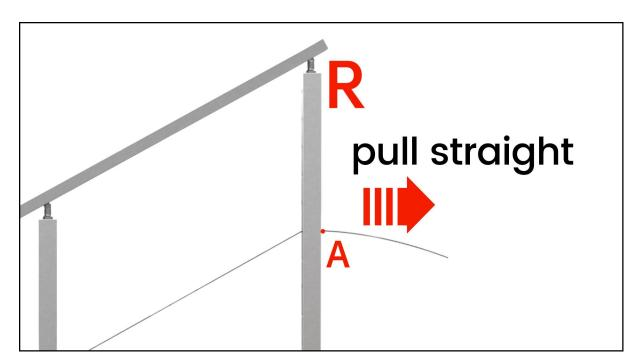
**Step 4 -** Pull the cable against the right end post, mark point A from the right side, and cut cable on point A with cable cutter **7**.
