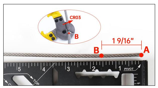
**Step 5 -** Mark and cut at B with cable cutter **7**, which is 1 9/16" away from point A.
