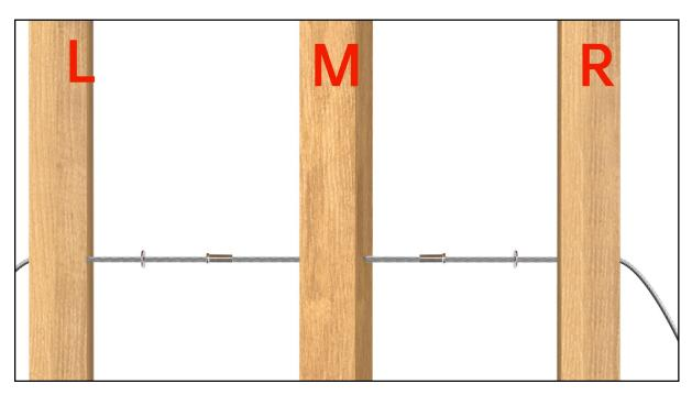
**Step 3 -** Put the adhesive washers **6** into the cable and pull the cable through all intermediates posts and level protector sleeves **6**.
