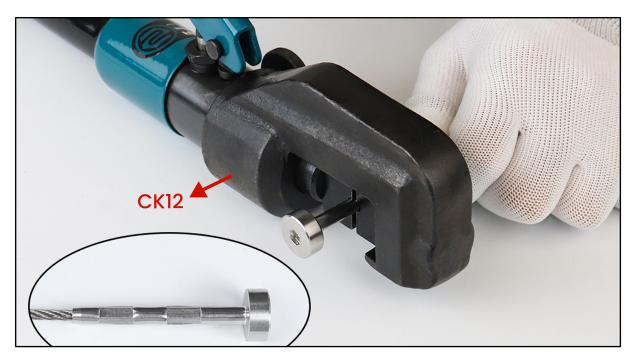
**Step 2 -** Swage the fixed end **2** with the hydraulic crimper **8**.
