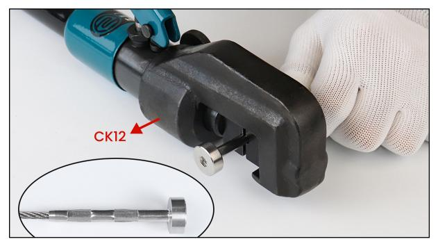
**Step 4 -** Swage the fixed end **2** with the hydraulic crimper **6**.
