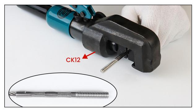
**Step 6 -** Swage tensioner **1** with hydraulic crimper **8**.
