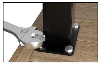
**Step 5 -** Thread the four screws **8** through the washer **9** and tighten them with a wrench.
