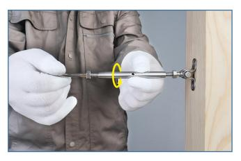
**Step 8 -** Loosen tensioner **1** to extend the turnbuckle to about 3/4.
