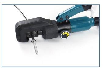
**Step 10 -** Crimp the right end of cable with the CK07 tensioner by crimper 7.
