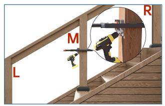
Step 1 - Locate hole positions with drill guide 3 and drill holes with drill bit 5 on all intermediate posts for cable to go through.
