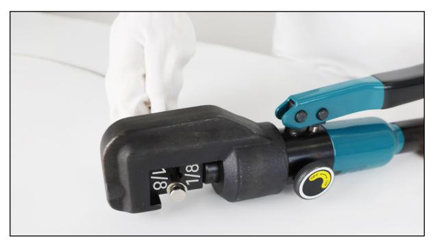
**Step 4 –** Swage the fixed end **2** with the hydraulic crimper tool **4**.
