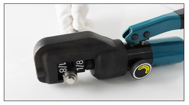
Step 4 - Put in angle washer 7 to the fixed end 2 and swage the fixed end with the hydraulic crimpe 4.
