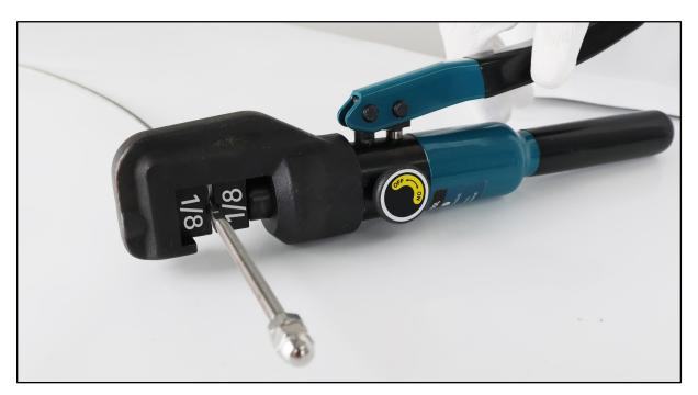
**Step 8 –** Swage tensioner **1** with the hydraulic crimper **4**.
