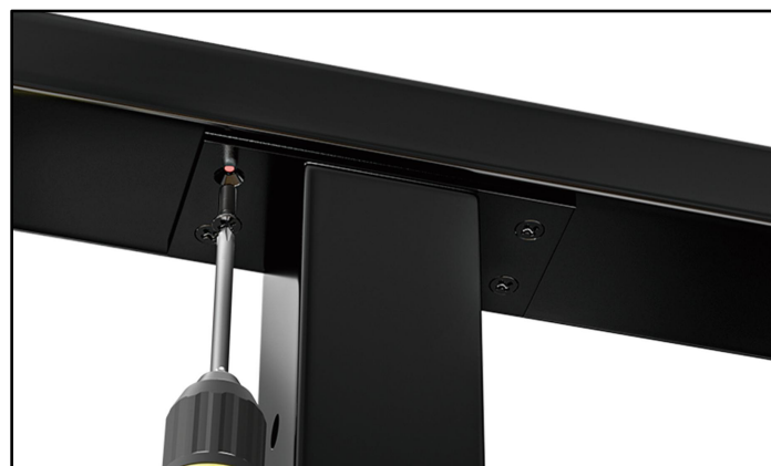
Step 4 - Install the handrails on posts with M5x16mm bolts.
