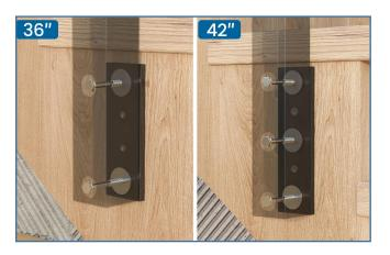
**Step 7 -** Insert M8 lag screws **9** through the post **1** and the spacer **8** into pilot holes.
