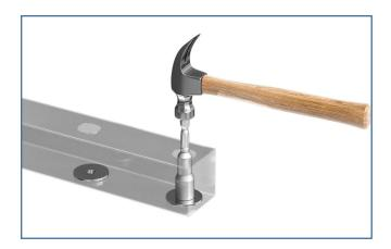
**Step 5 -** Install the washer **7** into the post **1** from the inside.
