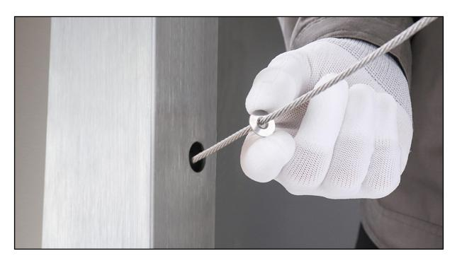
**Step 8 -** Install adhesive washers **6** and angle protector sleeves **6**.
