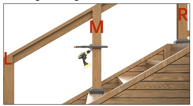
**Step 1 –** Locate hole positions and drill 30 degrees through holes with drill guide **8** on all intermediate posts with a 5/16" drill bit.
