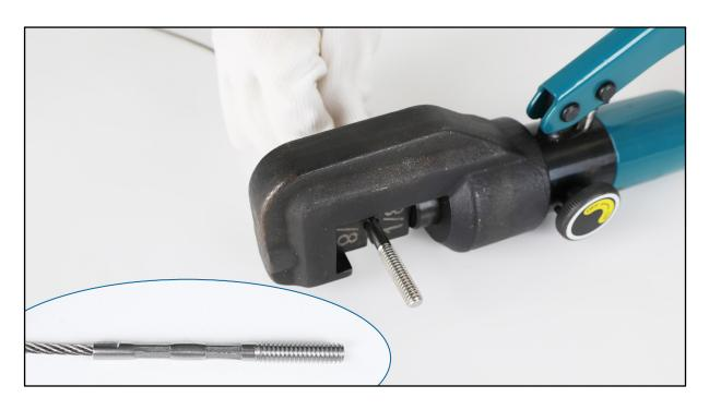
**Step 2 -** Put angle washer **7** into the fixed end **1** before swaging with hydraulic crimper **8**.
