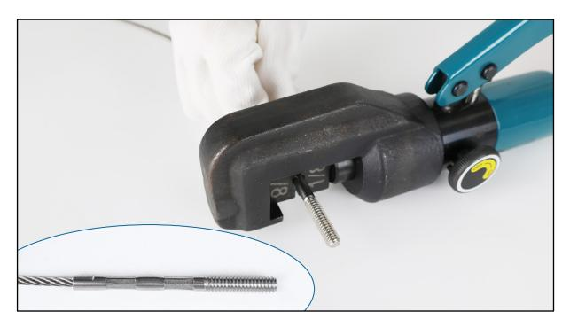
**Step 8 -** Swage tensioner **1** with the hydraulic crimper **9**.
