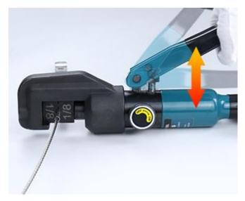
**Step 3** - Press the handles repeatedly until the terminal is fully swaged.
