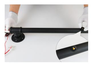
**Step 2 -** Install two LED lights 13 to the handrail tubes 11 and pull two I+ wires near the 3rd terminal 15.
