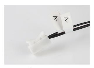
**Step 3 -** Install two A- to one side of the 2rd terminal **15**.
