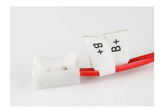
**Step 4** - Install two B+ to one side of the 3rd terminal **(b)**.
