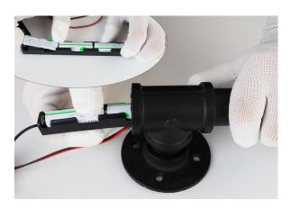
**Step 3** - Install the battery 18 into the battery holder and insert it into the handrail tube 1.
