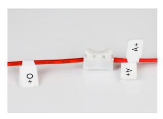
**Step 2 -** Install O+ to another side of the 1st terminal **(b)**.
