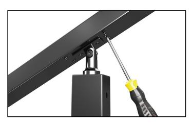
**Step 3 -** Install the M5x14mm bolts.
