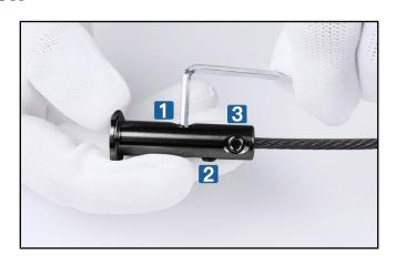
**Step 2 -** Put the cable **6** into the fixed end **5** and tighten the set screws in sequence with the 2.5mm Allen wrench.
