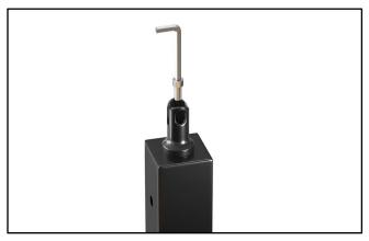
**Step 1 -** Install the bracket base 12 to the post 10 with 5mm Allen wrench.
