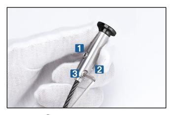
**Step 6** – Put the cable into the tensioner 14 and tighten the set screws in sequence with 2.5mm Allen wrench.
