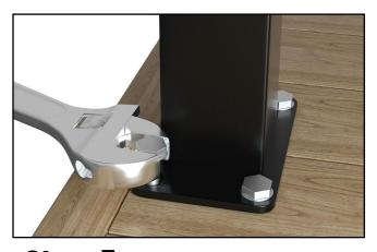
**Step 5 -** Thread four screws through the washer and tighten them with a wrench.
