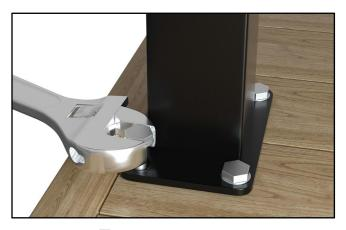
**Step 5 -** Thread the four screws through the washer and tighten them with a wrench.
