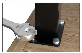
**Step 5 -** Thread the four screws 2 through the washer and tighten them with a wrench.
