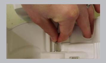
Push the coupling into the connection while maintaining your grasp on the metal ring.
