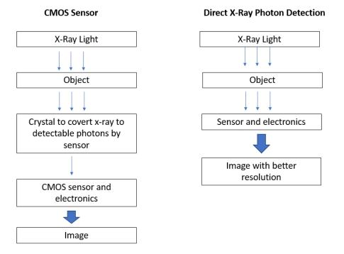
DXPD technology provides better image resolution compared to CMOS technology due to reduced loss of photons in the imaging process.
